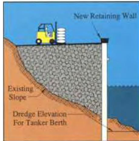
**Figure 2: Expanded shale used as retaining wall backfill (ECSI, 2013)**
