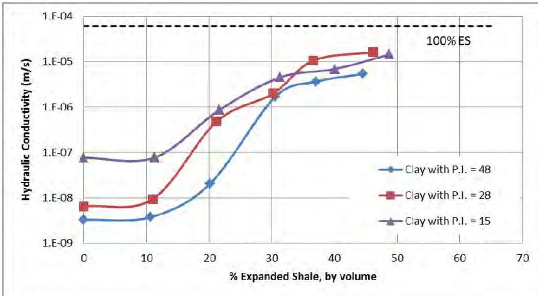
Figure 8: Effect of expanded shale amendment on hydraulic conductivity of clays for reduced proctor effort
