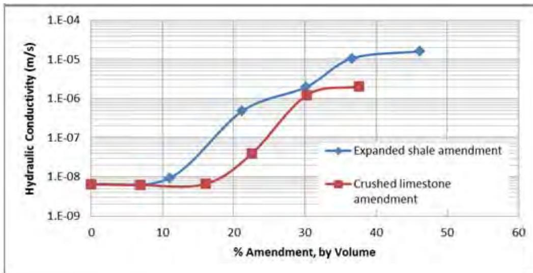
**Figure 10: Effect of expanded shale and crushed limestone amendment on hydraulic conductivity of clay with P.I. of 28**
