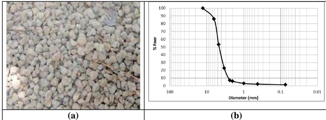
**Figure 4: Expanded Shale Lightweight Aggregate**
