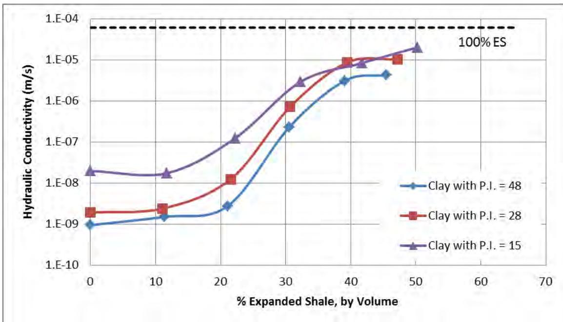
Figure 9: Effect of expanded shale amendment on hydraulic conductivity of clays for reduced proctor effort
