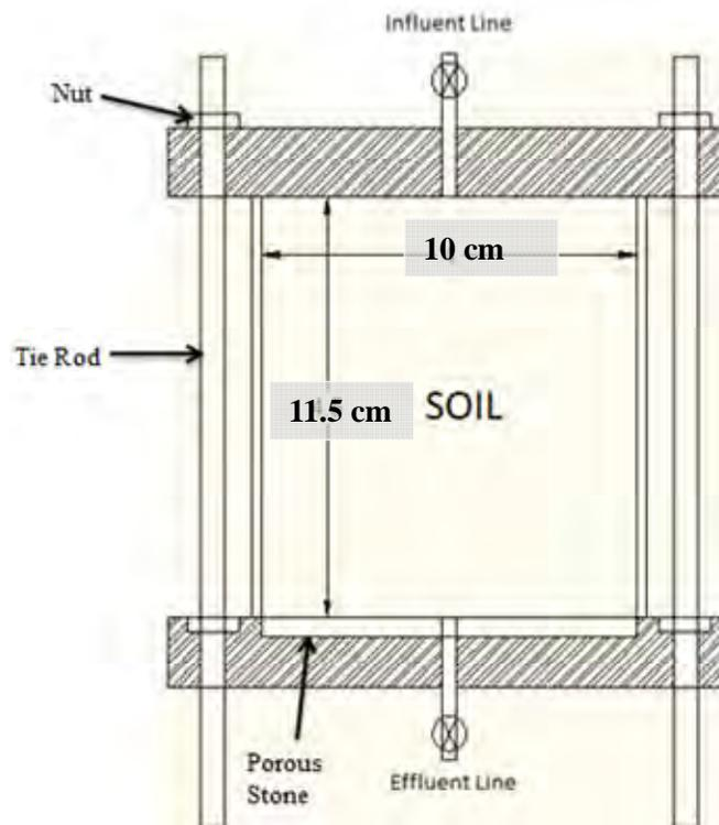
**Figure 5: Schematic of the compaction-mold permeameter**
