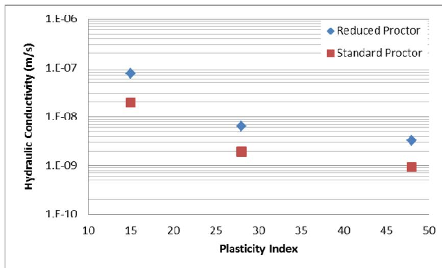
**Figure 7: Variation of hydraulic conductivity with plasticity index for non-amended clayey soils**
