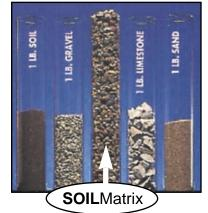
Tubes containing equal weights of soil, gravel, SOILMatrix, limestone and sand to demonstrate the difference in relative volume.
