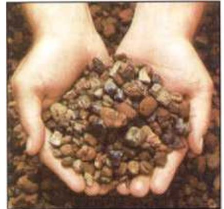
The strength of ESCS aggregates aids the SmartWall CMU's chipping resistance.
