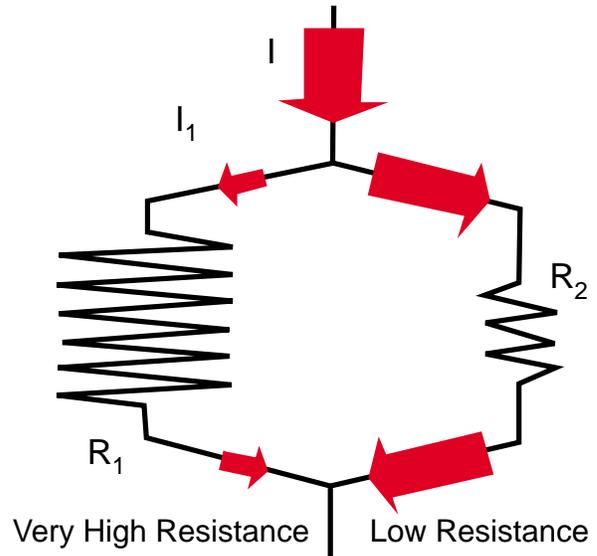
*Figure 1. Current flow in an electric network*
