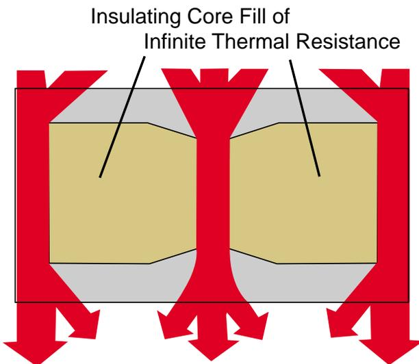
*Figure 2. Heat flow in an insulated concrete masonry unit*
